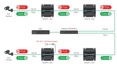
Transmission distance may vary depending on the type and quality of cable, use of power and environmental condition.
